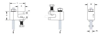
Material: Cast iron Finish: Electro-galvanized
