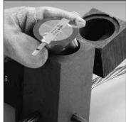
Insert CADWELD PLUS package into mold (may require use of a cover/baffle)
