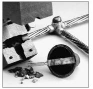
Open the mold and remove the expended steel cup - no special disposal required
