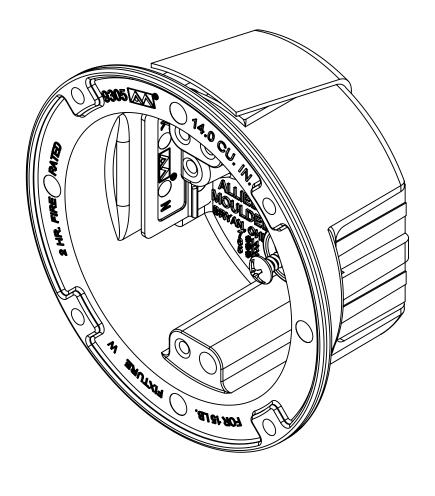
1.) BOX MATERIAL: FIBERGLASS REINFORCED POLYESTER, SNAP BRACKET MATERIAL: GALVANIZED STEEL, SNAP BRACKET SCREW MATERIAL: ZINC PLATED STEEL, SPEED KLAMP MATERIAL: PVC
