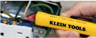
The NCVT-1 detects standard voltage (48-1000V AC) in cables, cords, circuit breakers, lighting fixtures, switches, outlets and wires.
