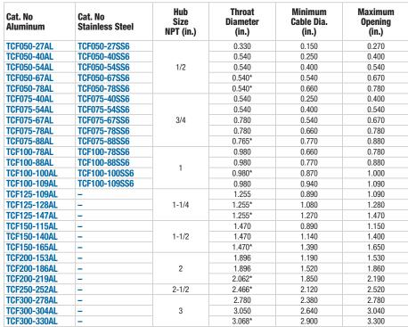
\*When cord will not fit through body, strip cord jacket and trim fillers if required. Insert cable ensuring the outer jacket reaches the end of the bushing as shown. Tighten gland nut onto body
