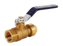
Push fit connect ends can be installed onto copper, PEX or CPVC. Insert stiffeners are included for use with PEX tubing. Configuration and Sizes: FNPT x PTC 1/2", 3/4", & 1". CWP 200 PSI. Third party certified no lead ANSI/NSF 61-G & DZR ANSI/NSF 14, IAPMO. ASSE 1061.
