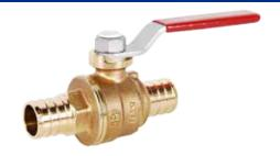
Maintenance-free dual Viton® O-ring stem seal, Dacromet® coated steel handle, CWP 400 PSI, ASTM F1806 PEX Ends. Third party certified no lead ANSI/NSF 61-G, NSF. Configuration and Sizes: PEX x PEX, 3/8"-1".
