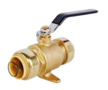
The P-2200NL Insta-Loc II™ drop ear ball valve stabilizes onto a frame or structure. Push fit connect ends can be installed onto copper, PEX or CPVC. Insert stiffeners are included for use with PEX tubing. Configuration and Sizes: PTC x PTC 1/2", 3/4", & 1". CWP 200 PSI. Third party certified no lead ANSI/NSF 61-G & DZR ANSI/NSF 14, IAPMO. ASSE 1061.
