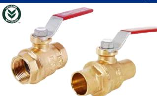
Maintenance-free, dual Viton® 0-ring stem design, lighter weight and durable forged no lead brass body, blow-out proof stem, PTFE seats for improved wear. Does not require any additional steps to solder, as compared to traditional brass valves. Suitable for potable water applications. 1/8" - 4", FNPT x FNPT and 1/2" - 4", Sweat x Sweat.
