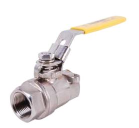
Heavy-duty two-piece investment cast body design, 316 stainless steel body & end adaptor. Bottom-loaded blowout-proof stem. Equipped with a latch-lock handle, 304 stainless steel trim, 316 stainless steel stem and ball. Ideal for commercial and industrial applications. Integral, tapped mounting pad for actuation or panel attachment. Sizes 2-1/2"- 4" are equipped with dual mounting pads. Available in sizes & configurations: 1/4"- 4", FNPT x FNPT.
