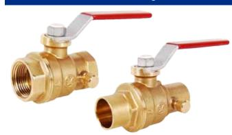
Maintenance-free, dual Viton® O-ring stem design, light weight and durable forged traditional brass body, blow-out proof stem, PTFE seats for improved wear. Ball with drain for maintenance or to prevent freeze. Dacromet® coated steel handle and nut for greater corrosion resistance. Available in sizes and configurations 1/2"-1", FNPT x FNPT and 1/2"-1", Sweat x Sweat.
