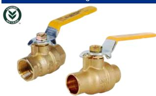
Forged no lead brass full port ball valve, bottom load blow-out proof stem with PTFE packing gland and nut. Constructed of no lead binary brass alloy. Suitable for potable water applications. Does not require any additional steps to solder, as compared to traditional brass valves. Available in sizes and configurations 1/4"- 3", FNPT x FNPT and 3/8"- 3", Sweat x Sweat.
