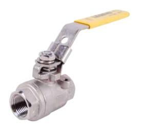
Heavy-duty two-piece investment cast body design, 316 stainless steel body & end adaptor. Bottom-loaded blowout-proof stem. Equipped with a latch-lock handle, 304 stainless steel trim, 316 stainless steel stem and ball. Ideal for commercial and industrial applications. Fiber reinforced, graphite impregnated seats maintain their shape in high pressure service. Integral, tapped mounting pad for actuation or panel attachment. Available in sizes & configurations: 1/4"- 2", FNPT x FNPT.
