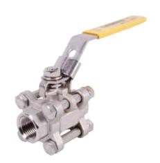
Heavy-duty three-piece investment cast body design, 316 stainless steel body & adaptors. Bottom-loaded blowout-proof stem. Equipped with a latch-lock handle, 304 stainless steel trim, 316 stainless steel stem and ball. Ideal for commercial and industrial applications. The body center section lifts or swings out to permit servicing without end adapter removal. Available in sizes & configurations: 1/4"- 2", FNPT x FNPT.
