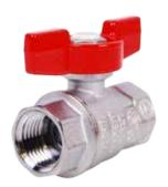
Maintenance-free, dual Viton® 0-ring stem design, light weight and durable forged traditional brass body, blow-out proof stem, PTFE seats for improved wear. Chrome plated forged brass. Coated cast aluminum tee handle that is lightweight and compact in size. Available in sizes and configurations 1/2"- 1", FNPT x FNPT.
