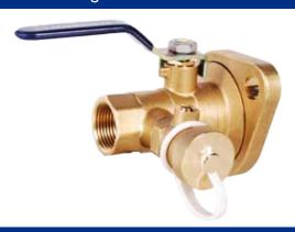
Traditional forged brass full port ball valve with flanged end and integrated drain valve for isolating circulator pumps. Standard flange connection rotates for positioning valve. Mounting holes are elongated to fit high velocity pumps. 1/4- turn tool activated drain valve with 3/4" GHT end and tethered brass cap. Configuration and Size: FNPT x Flange, Sweat x Flange, and 3/4", 1" and 1-1/4".
