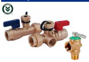
Hot and cold water heater isolation valves and pressure relief valve. No lead brass full port ball valves, include 150 PSI pressure relief valve. Tethered cap on tool activated drain valves integral in body of each valve, hot and cold. Configuration and Size: FNPT (Captive Union) X FNPT, Sweat (Captive Union) X Sweat, 3/4" x 3/4", & 1" x 1".
