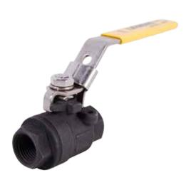
Heavy-duty two-piece carbon steel investment cast body design Bottom-loaded blowout-proof stem, 316 stainless steel ball and stem, 304 stainless steel latch-lock handle and trim. Fiber reinforced graphite impregnated seats maintain their shape in high pressure service. Integral, tapped mounting pad for actuation or panel attachment. Ideal for commercial or industrial applications. Available in sizes & configurations: 1/4"- 2", FNPT x FNPT.
