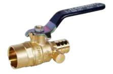
Maintenance-free dual EPDM® 0-ring stem seal, zinc plated steel handle with vinyl sleeve CWP 400 PSI, with drain. Third Party certified no lead ANSI/NSF 61-G & DZR ANSI/NSF 14, IAPMO. ASTM F1806. Configuration and Sizes: Sweat x PEX, 1/2"-1".
