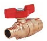
Maintenance-free dual Viton® O-ring stem seal, coated cast aluminum handle, CWP 400 PSI, ASTM F1806. With coated cast aluminum tee handle. Third party certified no lead ANSI/NSF 61-G, NSF. Configuration and Sizes: MNPT x PEX, 1/2" & 3/4".
