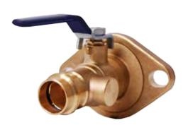
LegendPress<sup>TM</sup> press fitting end traditional forged brass full port ball valve with flanged end connection for isolating circulator pumps. Mounting holes are elongated to fit high velocity pumps. Standard flange connection rotates for positioning valve. Configuration and Size: Press Fitting x Flange, 3/4", 1" and 1-1/4".
