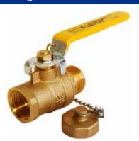
Traditional forged brass full port ball valve, 3/4" FNPT x 3/4" GHT. Garden hose includes GHT cap with gasket and tethered to valve end. \*Capped GHT connection is rated 125 PSI.
