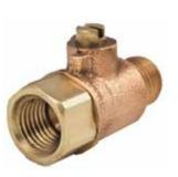
No lead cast brass test cock ball valve, with screwdriver slot stem for actuation. Configurations and Sizes: FNPT x MNPT,( 1/4" x 1/8") & (1/4"x 1/4").
