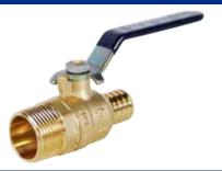
Maintenance-free dual EPDM® 0-ring stem seal, zinc plated steel handle with vinyl sleeve. Third Party certified no lead ANSI/NSF 61-G & DZR ANSI/NSF 14, IAPMO. CWP 400 PSI. ASTM F1806. Configuration and Sizes: MNPT x PEX, 1/2"-1".
