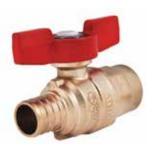
Maintenance-free dual Viton® 0-ring stem seal, coated cast aluminum handle, CWP 400 PSI, ASTM F1806 PEX Ends. With coated cast aluminum tee handle. Third party certified no lead ANSI/NSF 61-G, NSF. Configuration and Sizes: Sweat x PEX, 1/2" & 3/4".
