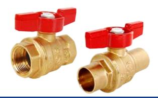
Maintenance-free, dual Viton® 0-ring stem design, lighter weight and durable forged traditional brass body, blow-out proof stem, PTFE seats for improved wear. Coated cast aluminum tee handle that is light weight and compact in size. Available in sizes and configurations 1/2" x 1", FNPT x FNPT and 1/2"-1", Sweat x Sweat.
