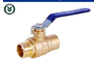
No lead forged brass full port ball valve for transitioning from a tank or boiler directly to copper tube. Configuration and Size: MNPT x Sweat, 3/4" x 3/4".
