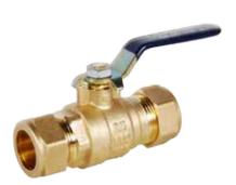
Full port ball valve with compression ends for convenient installation onto copper tubing. Constructed of no lead binary brass. Configuration and Sizes: Compression x Compression, 1/2", 3/4", & 1". Third party certified no lead ANSI/NSF 61-G, IAPMO.
