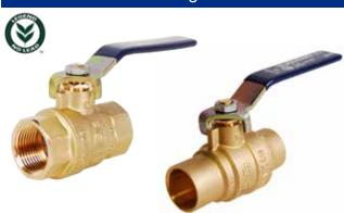
The T/S-2000NL no lead brass full port ball valve has a larger pattern body suitable for most any application. Constructed of no lead & DZR binary brass alloy. Available in sizes and configurations 1/4"-4", FNPT x FNPT and 1/2"-4", Sweat x Sweat.
