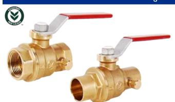
Maintenance-free, dual Viton® 0-ring stem design, light weight and durable forged no lead brass body, blow-out proof stem, PTFE seats for improved wear. Ball with drain for maintenance or to prevent freeze. Dacromet® coated steel handle and nut for greater corrosion resistance. Constructed of no lead binary brass alloy. Suitable for potable water applications. Available in sizes and configurations 1/2"-1", FNPT x FNPT and 1/2"-1", Sweat x Sweat.
