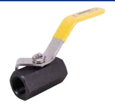
Heavy-duty one-piece carbon steel barstock body. Bottom-loaded blowout-proof stem, 304 stainless steel handle & nut, stem and ball. Ideal for commercial or industrial applications where port size is not critical. Available in sizes and configurations 1/4" - 2", FNPT x FNPT.
