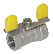
One-piece cast 316 stainless steel body, 304 stainless steel T-handle. 316 stainless steel stem and ball. Available in 1/4" FNPT x FNPT.
