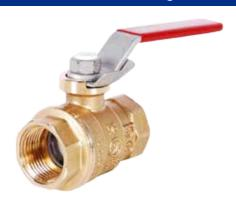
Maintenance-free, dual Viton® 0-ring stem design, lighter weight and durable forged traditional brass body, blow-out proof stem, PTFE seats for improved wear. Dacromet® coated steel handle and nut for greater corrosion resistance with Dacromet® coated steel lock shield that includes eyelet for padlock. Available in sizes and configurations 1/2"- 2", FNPT x FNPT.
