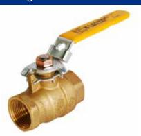
Traditional brass full port ball valve, bottom-loaded blow-out proof stem with PTFE packing gland and nut, 304 stainless steel ball and stem which are stronger and ideal for more heavy use, more frequent operation. Chrome plated steel handle with locking mechanism, eyelet for padlock. Available in sizes and configurations 1/2"- 2", FNPT x FNPT.
