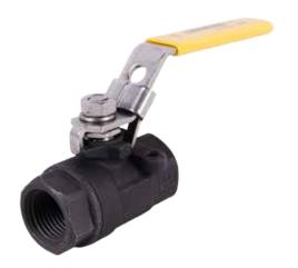
Heavy-duty two-piece carbon steel investment cast body and end adaptor. Bottom-loaded blowout-proof stem, 316 stainless steel ball and stem, 304 stainless steel latch-lock handle and trim. Fiber reinforced graphite impregnated seats maintain their shape in high pressure service. Integral, tapped mounting pad for actuation or panel attachment. Ideal for commercial or industrial applications. Available in sizes & configurations: 1/4" - 2", FNPT x FNPT.
