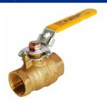
Traditional brass full port ball valve, bottom-loaded blow-out proof stem with PTFE packing gland and nut. Chrome plated steel handle with locking mechanism, eyelet for padlock. Available in sizes and configurations 1/4" - 2", FNPT x FNPT.
