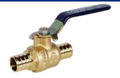
Maintenance-free dual EPDM® 0-ring stem seal, zinc plated steel handle with vinyl cover CWP 400 PSI, ASTM F1806. Third party certified no lead ANSI/NSF 61-G & ANSI/NSF 14, IAPMO. Configuration and Sizes: PEX x DZR PEX, 1/2"-1-1/4".
