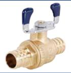
Maintenance-free dual EPDM® O-ring stem seal, zinc plated steel tee handle, CWP 400 PSI, Third Party certified no lead ASNI/NSF 61-G & DZR ANSI/NSF 14, IAPMO. ASTM F1806. Configuration and Sizes: PEX x PEX, 1/2"-3/4".
