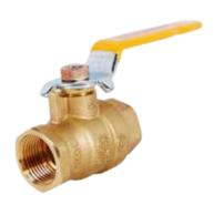
Traditional brass full port ball valve, bottom-loaded blow-out proof stem with PTFE packing gland and nut. 304 stainless steel ball and stem which are stronger and ideal for more heavy use, more frequent operation. Available in sizes and configurations 1/2"- 2", FNPT x FNPT.
