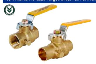
Forged no lead brass full port ball valve, bottom load blow-out proof stem with PTFE packing gland and nut. Drain for maintenance and freeze protection. Constructed of no lead binary brass alloy. Does not require any additional steps to solder, as compared to traditional brass valves. Suitable for potable water applications. Available in sizes and configurations 1/2"- 1", FNPT x FNPT and 1/2"- 1", Sweat x Sweat.
