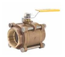
Large pattern three-piece cast bronze body and end adapters. Blow-out proof, forged brass stem. Chrome plated cast brass ball. PTFE seats (2), end adapter seals (2), stem seal, and stem packing. Packing nut is forged brass. Chrome plated steel handle with vinyl sleeve. AISI 304 stainless steel bolts, split washers and nuts (4 each).
