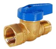
T-3000 Blue Top One-Piece Forged Brass Gas Ball Valve Flare x FNPT (3/8" x 1/2", 1/2", 1/2" x 3/4", 5/8" (15/16-16) x 1/2", 5/8" (7/8-14) x 3/4", 5/8" (15/16-16) x 3/4")
