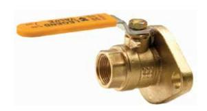
Traditional forged brass full port ball valve with flanged end for isolating circulator pumps. Configuration and Size: FNPT x Flange, Sweat x Flange, and 3/4", 1" and 1-1/4".
