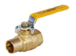
Traditional forged brass full port ball valve for connecting boilers to copper tube. Configurations and Sizes: FNPT x Sweat, 1/2"-1".
