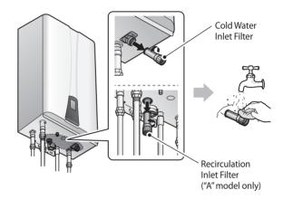
3. Reinsert and tighten the filters.
