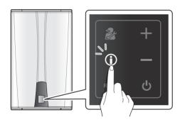
Press the + or – buttons to switch between the information types.
