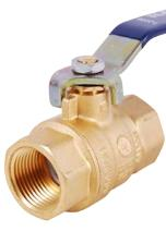
The T-2000 Series ball valve has a dual seal: PTFE packing and an EPDM O-ring stem seal. Full Port, forged brass body, end adapter, and ball. The T-2000 is a larger body ball valve, meeting MSS SP-110. It is manufactured in an ISO Certified facility utilizing automation and comprehensive TQM programs. Each valve is 100% factory pressure tested. Zinc plated handle and nut for greater corrosion resistance.
