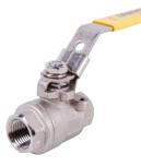
Large port ball valve; two-piece, 316 stainless steel investment casting; bottom-load blow-out proof stem; latch-lock handle; reinforced graphite impregnated seats; integral, tapped mounting pad for actuation or panel attachment.
