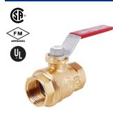
Maintenance free, dual Viton® O-ring stem design, lighter weight and durable forged body, blow out proof stem, TFM-PTFE® seats for improved wear. Dacromet® coated steel handle and nut for greater corrosion resistance. Each valve is 100% factory pressure tested.
