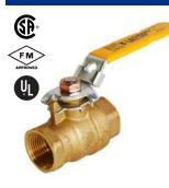
Full port ball valve with stainless steel ball and stem for greater strength, intended for frequent actuation. Includes latch lock steel handle and trim. Lockable in the full open and fully close positions.
