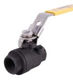
Two-piece, carbon steel investment casting; bottom-load blow-out proof stem; latch-lock handle; reinforced graphite impregnated seats; integral, tapped mounting pad for actuation or panel attachment.
