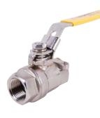
Full port ball valve; two-piece, 316 stainless steel investment casting; bottom-load blow-out proof stem; latch-lock handle; integral, tapped mounting pad for actuation or panel attachment.
