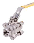
Full port ball valve; heavy-duty, three-piece 316 stainless steel investment casting; bottom-load blow-out proof stem; latch-lock handle; four 304 stainless steel nuts and bolts; body center lifts or swings out to permit servicing without end adapter removal.
