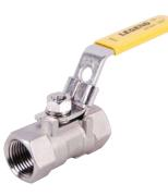
Reduced port ball valve; one-piece, 316 stainless steel investment casting; bottom-load blow-out proof stem; latch-lock handle; and ideal for commercial or industrial applications.
