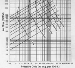
STRAIGHT RUN \* FD 72-R1 Test Code of the Air Diffusion Council. Friction loss is computed in inches of water gauge per 100 ft. of straight duct. By using CFM or FPM values for a given duct dimension, the friction loss can be determined. Conversion of CFM to FPM also can be made.
