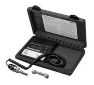
This portable, lightweight, solid state instrument indicates the vacuum pressure in the system using thermocouple technology. This is important because you need to know the vacuum to confirm moisture removal. The battery powered gauge measures atmospheric pressures of 760,000 to 1 micron in easy to read 1/2" high numbers (Part #69075).
